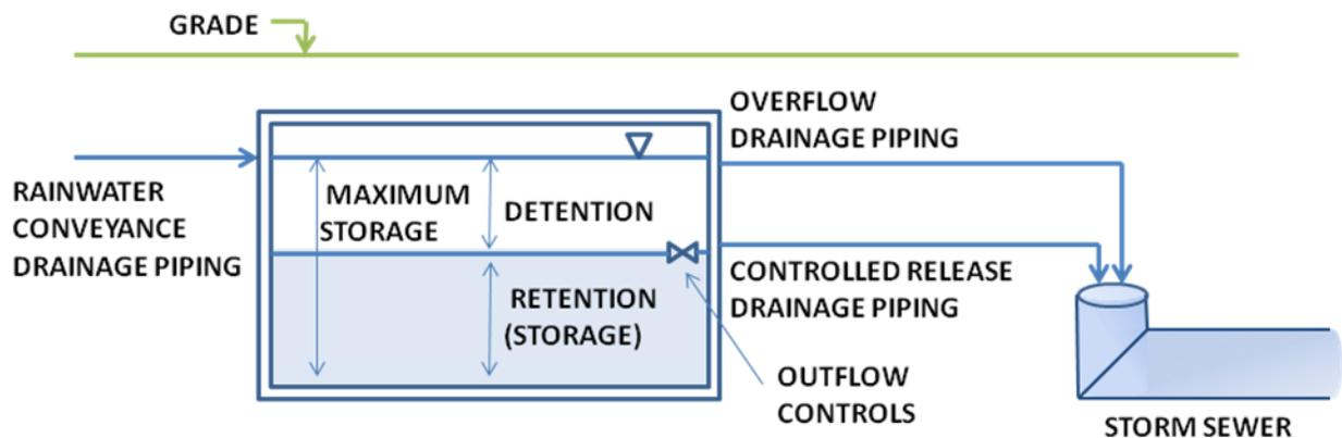
**Figure D-1. Schematic of RWH system with outflow controls and controlled release drainage piping for stormwater management. ('DETENTION' is the volume of runoff to be slowly released to storm sewer. The remaining volume 'RETENTION' is used to supply rainwater to permitted fixtures)**
