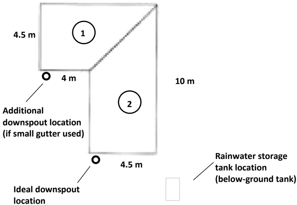
Figure A-2. Roof drainage area to be guttered (projected 'top-down' view)<sup>14</sup>
