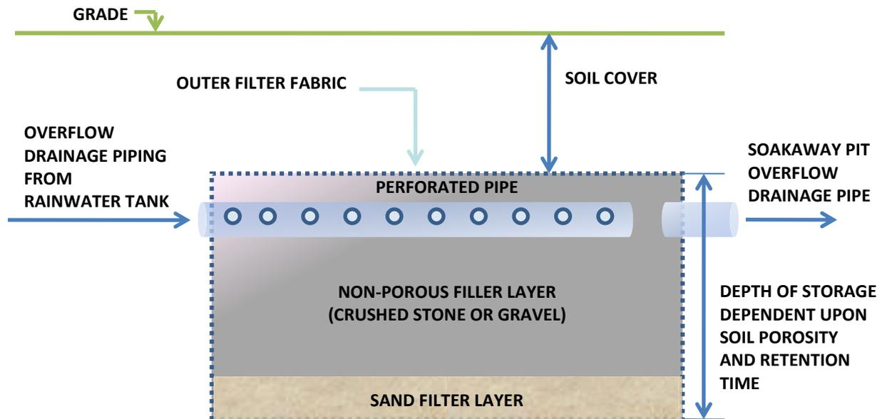
Figure D-2. Sketch of a typical soakaway pit (cross-section view)<sup>37</sup>
