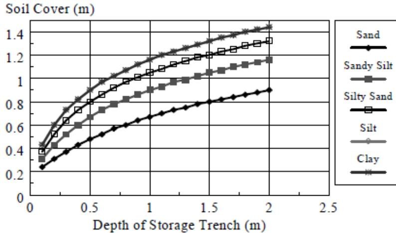
Figure D-3. Soil cover for soakaway pits, based on frost heave<sup>41</sup>
