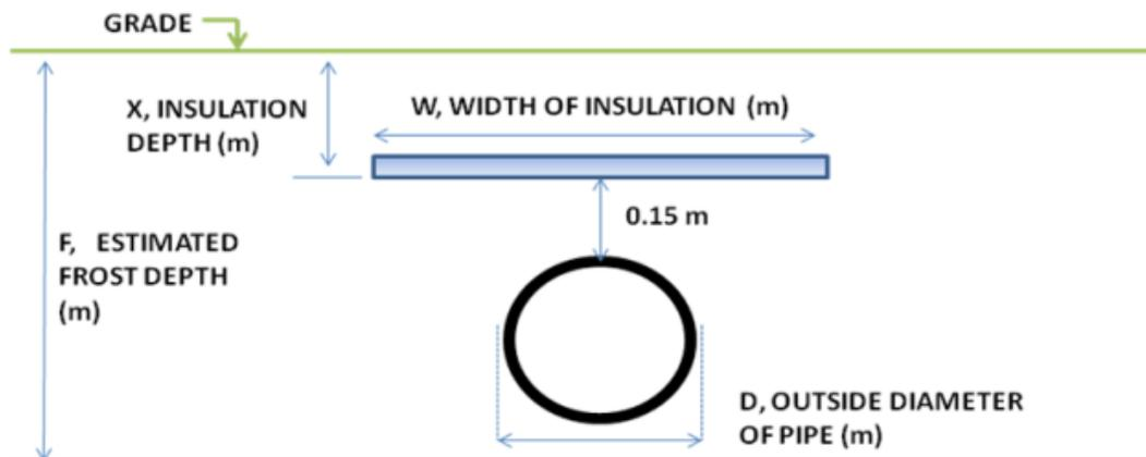
Figure A-5. Frost protection of pipe by horizontal insulation<sup>19</sup>
