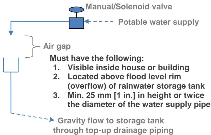
Figure 4-2. Schematic drawing of a top-up system with an air gap<sup>7</sup>
