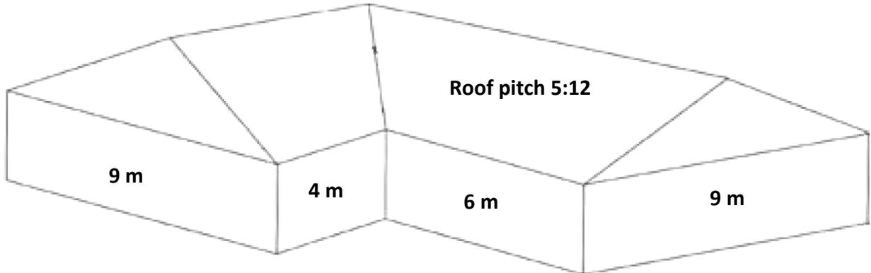
Figure A-1. Roof drainage area to be guttered (isometric 'facing' view)<sup>13</sup>
