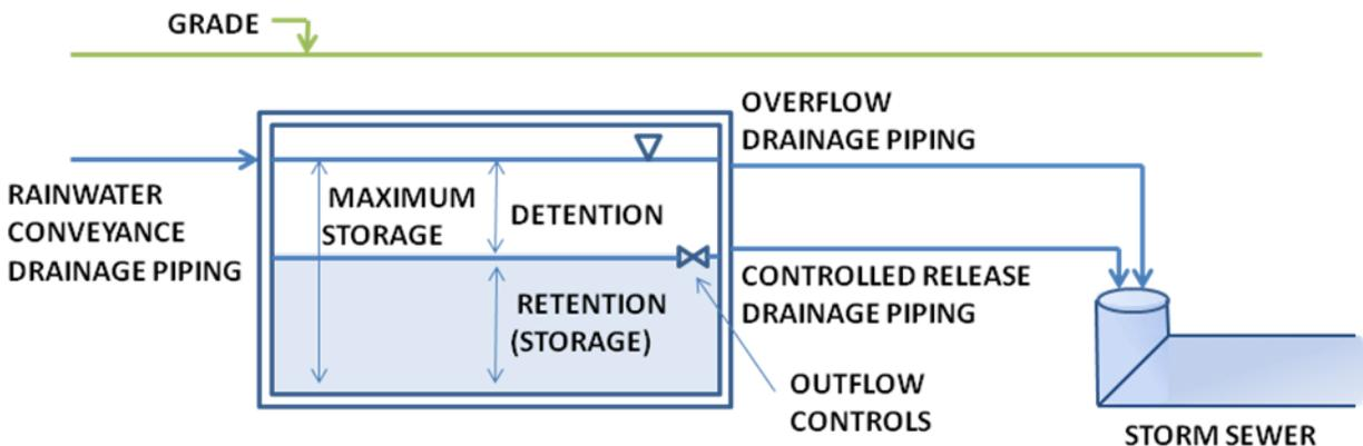
**Figure 6-1. Schematic of RWH system with outflow controls and controlled release drainage piping for stormwater management. ('DETENTION' is the volume of runoff to be slowly released to storm sewer. The remaining volume 'RETENTION' is used to supply rainwater to permitted fixtures**
